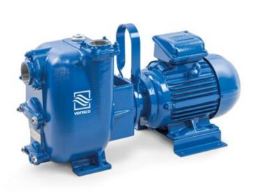
**Product Data** Suction port Threaded - 3" ISO 228 (BSP) Delivery port Threaded - 3" ISO 228 (BSP) Qmax 95 m<sup>3</sup>/h - 1583 l/min (418 USgpm) Hmax 16 m (52 ft) Solids handling 40 mm (1,5 ") Motor power 5,5 kW - 7,5 HP Motor type **IEC** standard Winding for inverters **Cast iron frame** Motor brand WEG W22 Premium Weight 112 ka
